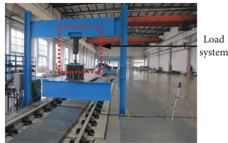
FIGURE 11: Quasi-static loading system.
