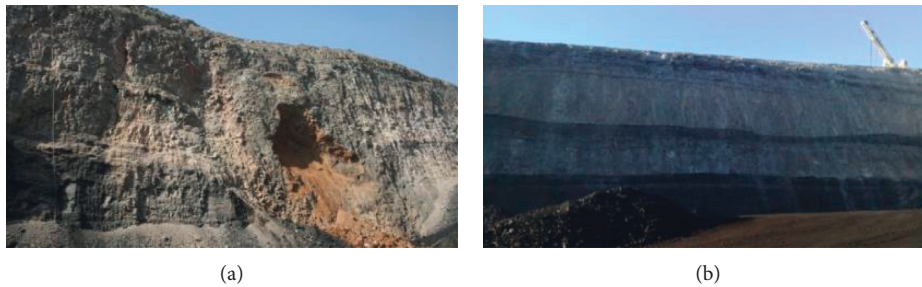
FIGURE 12: Presplit blasting effect. (a) Presplit face when S = 4.0 m and (b) presplit face when S = 3.4 m.
