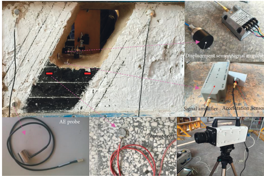
FIGURE 5: Monitoring equipment and layout.
