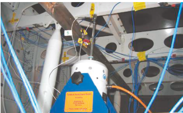
FIGURE 8: Internal transient impact load test process.
