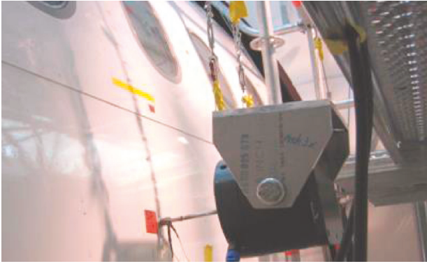
FIGURE 7: External transient impact load test process.
