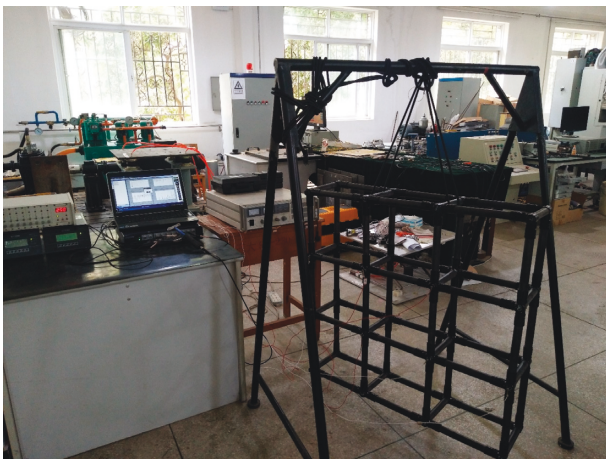
FIGURE 6: Modal experiment of CFRP truss.
