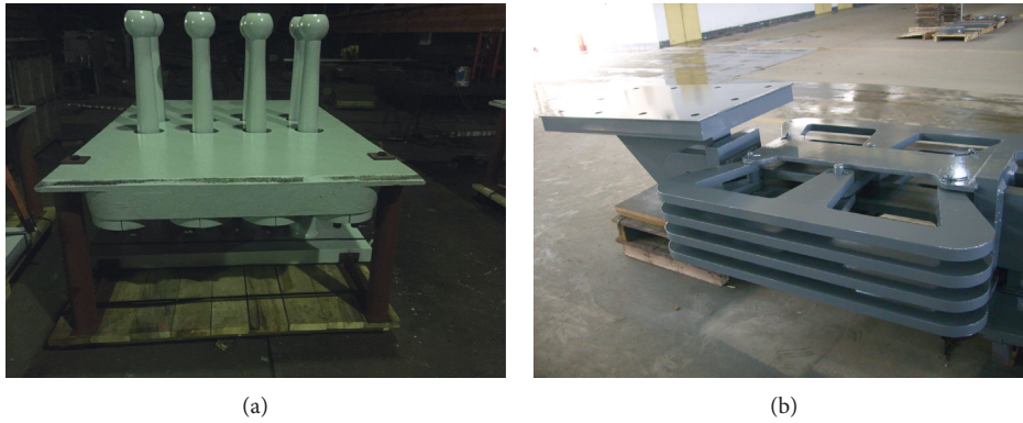
FIGURE 15: (a) Cylindrical and (b) E-shaped damping devices based on modular design.
