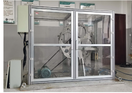
FIGURE 1: Prototype of the multiple impact equipment.
