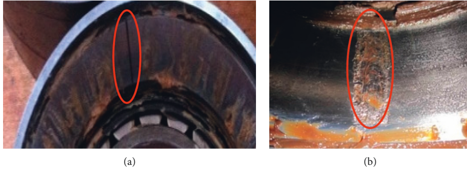
FIGURE 22: Photo of the faults (a) on the outer race and (b) on the inner race.
