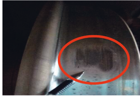
FIGURE 38: The defect on the tested wheel tread.
