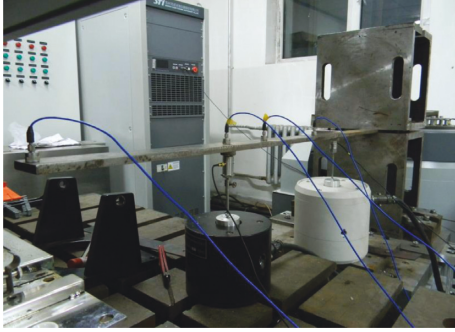
FIGURE 3: Photo of cantilever beam experiment setup.
