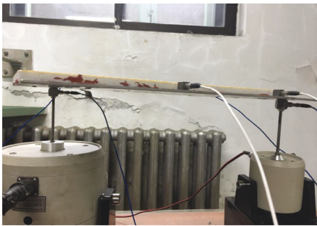
FIGURE 6: Photo of thermal protection composite plate experiment setup.
