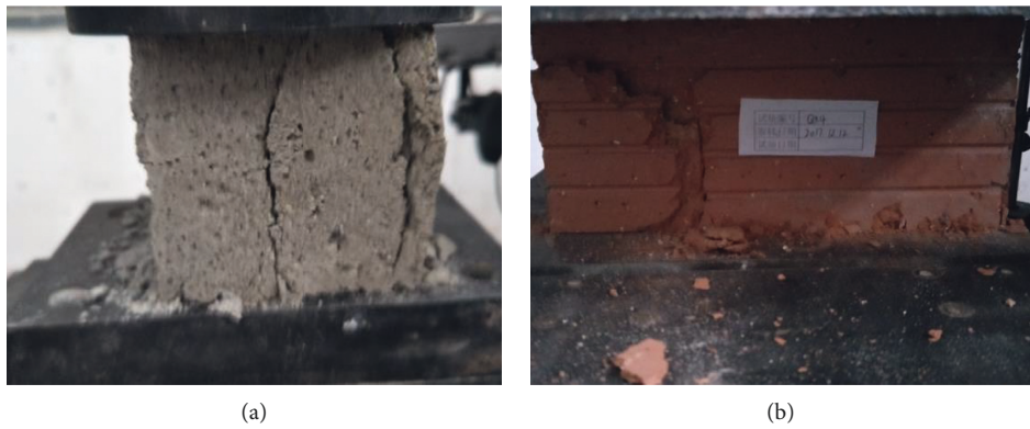
FIGURE 5: Material mechanical properties test. (a) Mortar mechanics test. (b) Mechanical properties test of sintered hollow brick.
