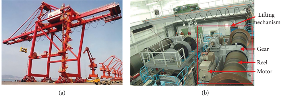
FIGURE 1: (a) Real map of quay crane and (b) its lifting mechanism.
