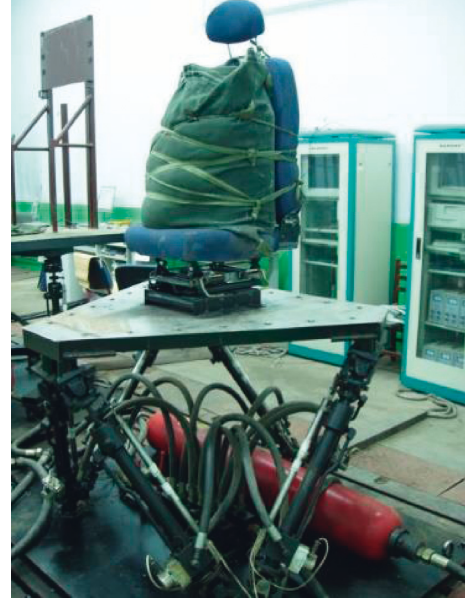
FIGURE 10: 6-DOF vibration representation test bed of a vehicle.
