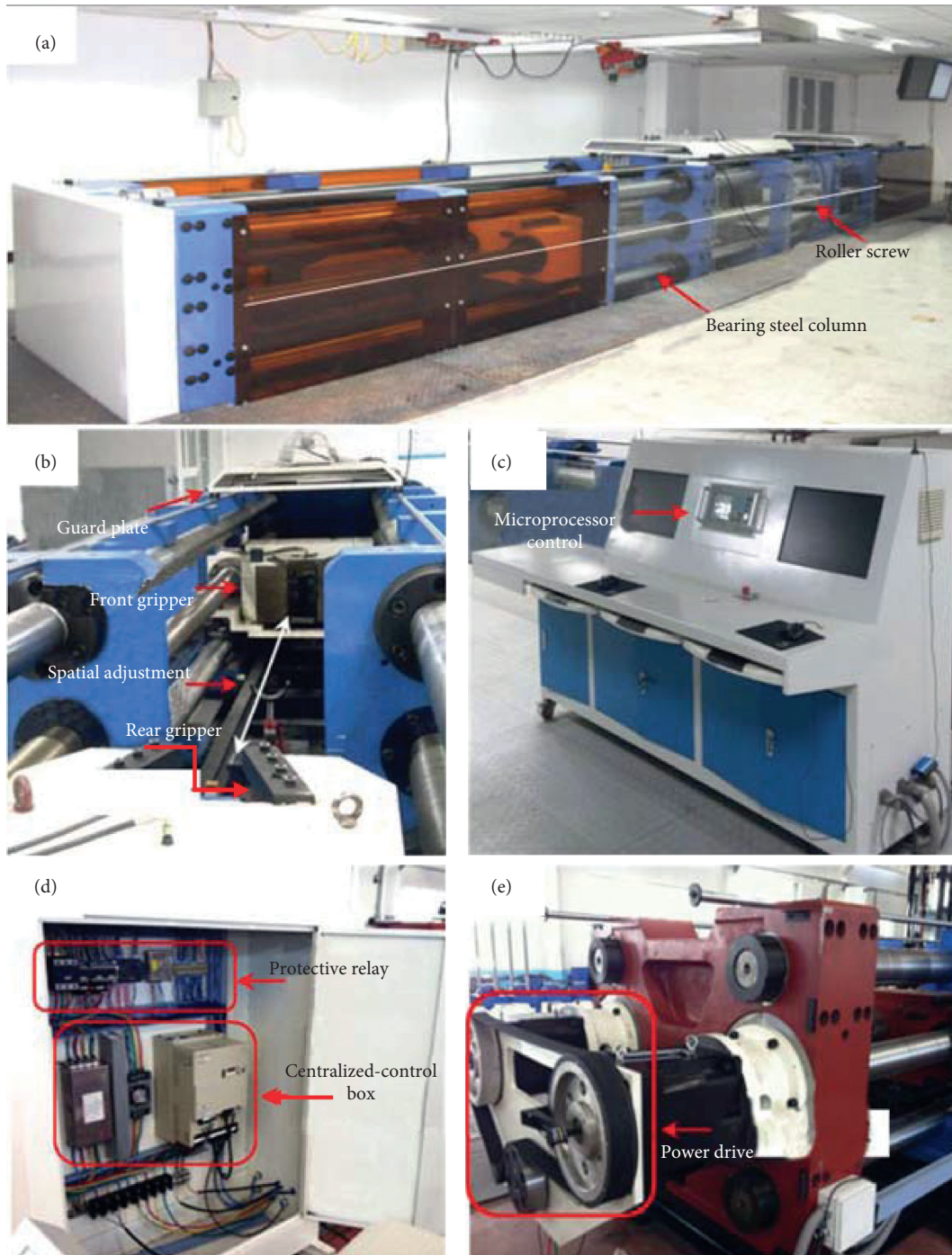
FIGURE 8: NPR anchor tensile testing machine: (a) host frame; (b) work platform; (c) experimental control system; (d) electrical control system; (e) motion transfer system.
