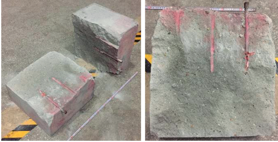
FIGURE 5: Overall morphology of the directional fracture surface.
