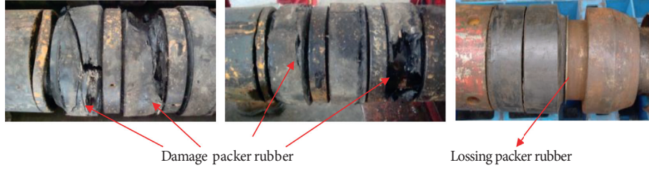
FIGURE 2: Failure cases of the rubber packer.
