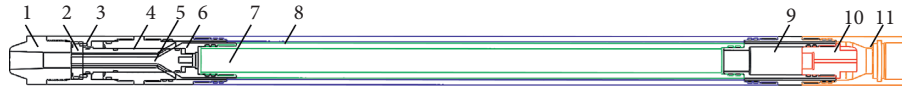
FIGURE 1: Mechanical structure of wireless control throttle. 1, inlet nozzle; 2, static flap; 3, adapter sleeve; 4, valve body; 5, dynamic flap; 6, adapter sleeve; 7, electric sealing cylinder; 8, air guide cylinder; 9, fixing frame; 10, head; 11, sleeve.
