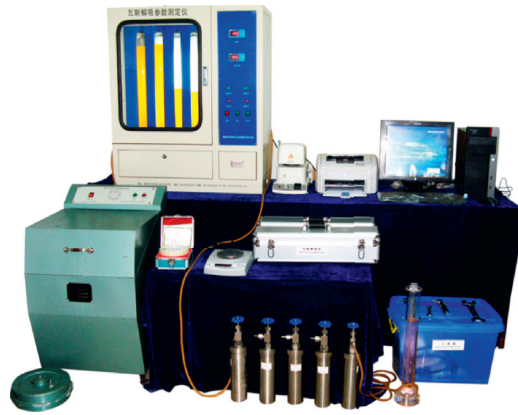
FIGURE 9: Direct measuring device for gas content.
