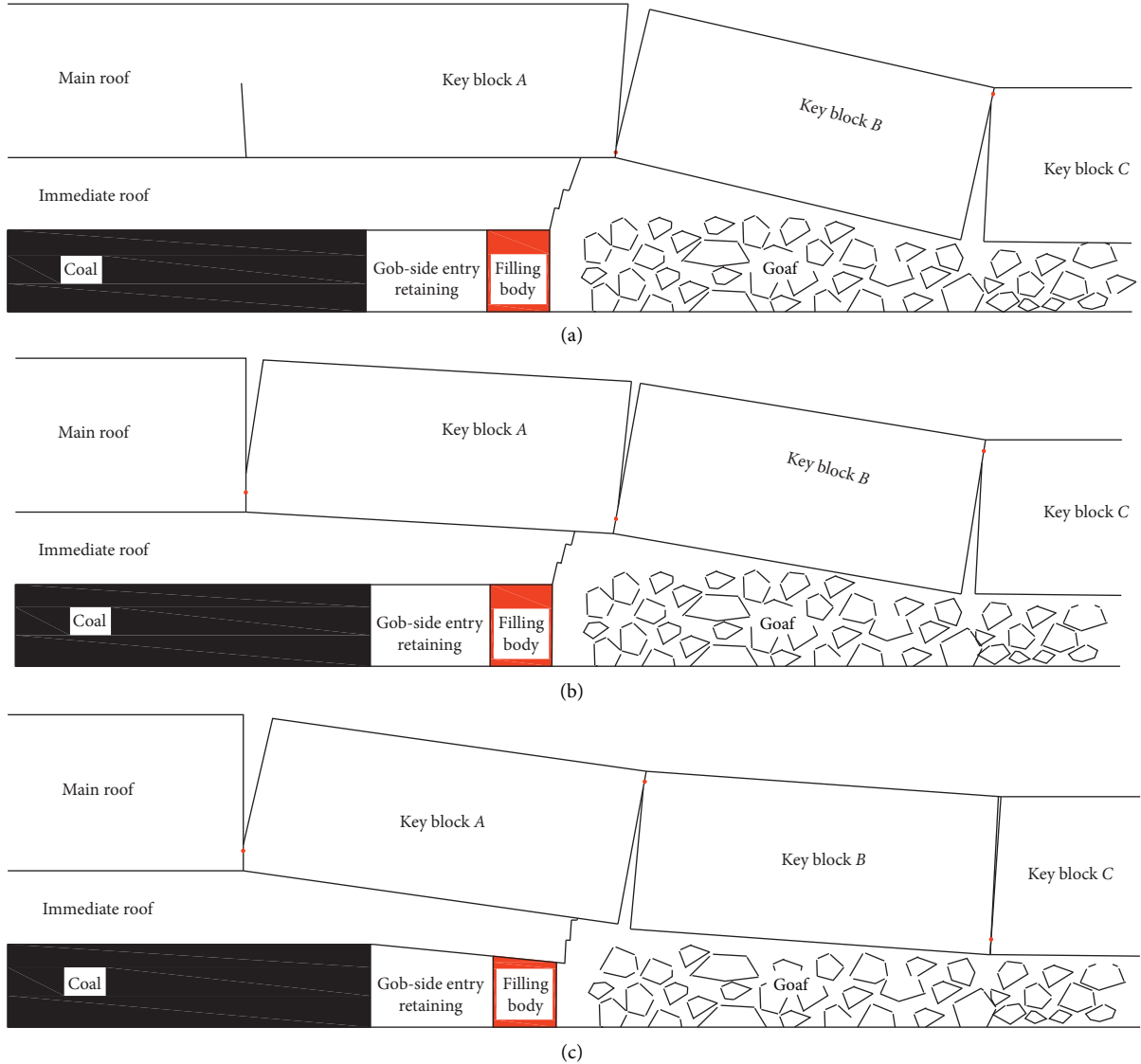
FIGURE 2: Structure form of short cantilever-articulated rock beam. (a) Roof structure in the stage of gob-side entry retaining, (b) roof structure in the early stage of reuse of gob-side entry retaining, and (c) the roof structure in the late stage of reuse of gob-side entry retaining.
