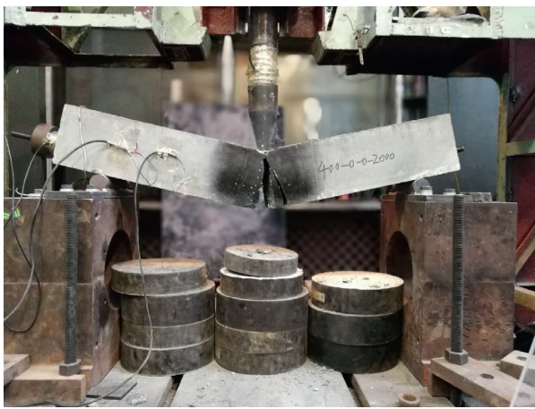
FIGURE 4: Typical deformation and failure characteristics of samples under impact load.
