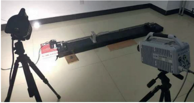
FIGURE 15: Impact characteristics experiment device for recoil spring.
