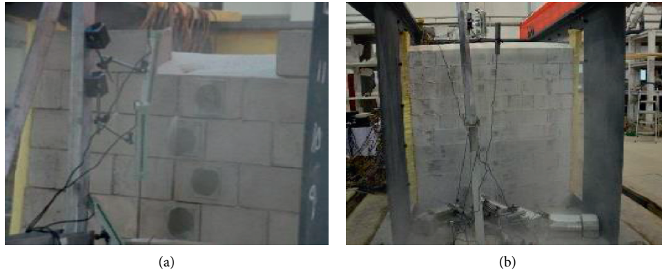
FIGURE 8: Seismic damage to RSRW. (a) Specimen 1 damage. (b) Specimen 2 damage.
