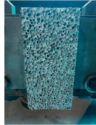
FIGURE 2: Closed-cell aluminum foam material.
