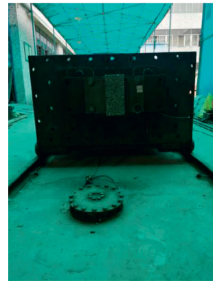
FIGURE 7: Horizontal traction impact test.
