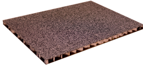
FIGURE 4: Experimental panel with speckle pattern.
