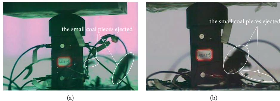
FIGURE 14: The ejection of small coals in the CGN1-1 and HSN2-3 during uniaxial compression tests: (a) CGN1-1, (b) HSN2-3.
