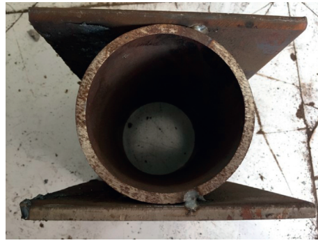
FIGURE 9: Specimen for compression test of steel tube.
