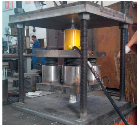
FIGURE 2: Field test diagram of uniaxial energy storage loading device.
