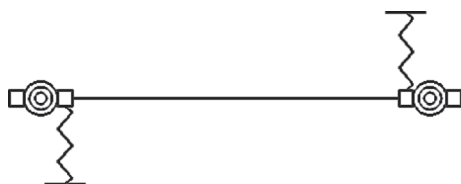
FIGURE 15: Schematic model of link beams in eccentric frames.
