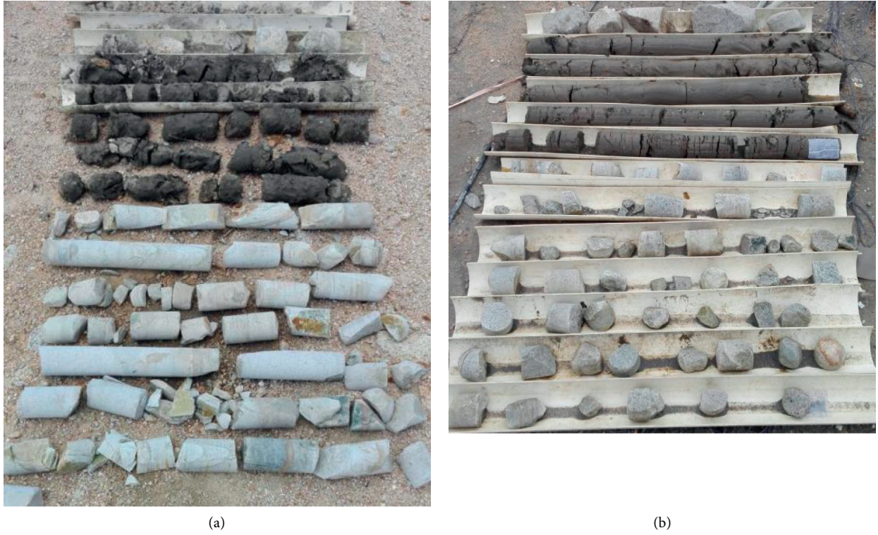
FIGURE 3: Rock cores (a) before blasting and (b) after blasting.
