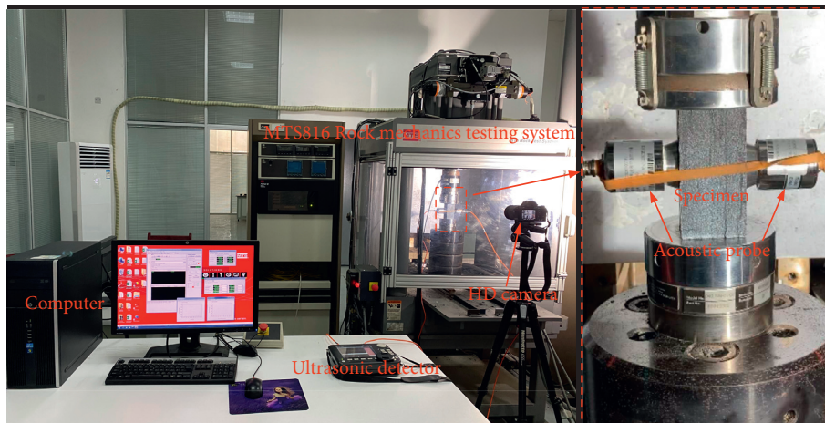
FIGURE 2: Test equipment and its installation and layout.
