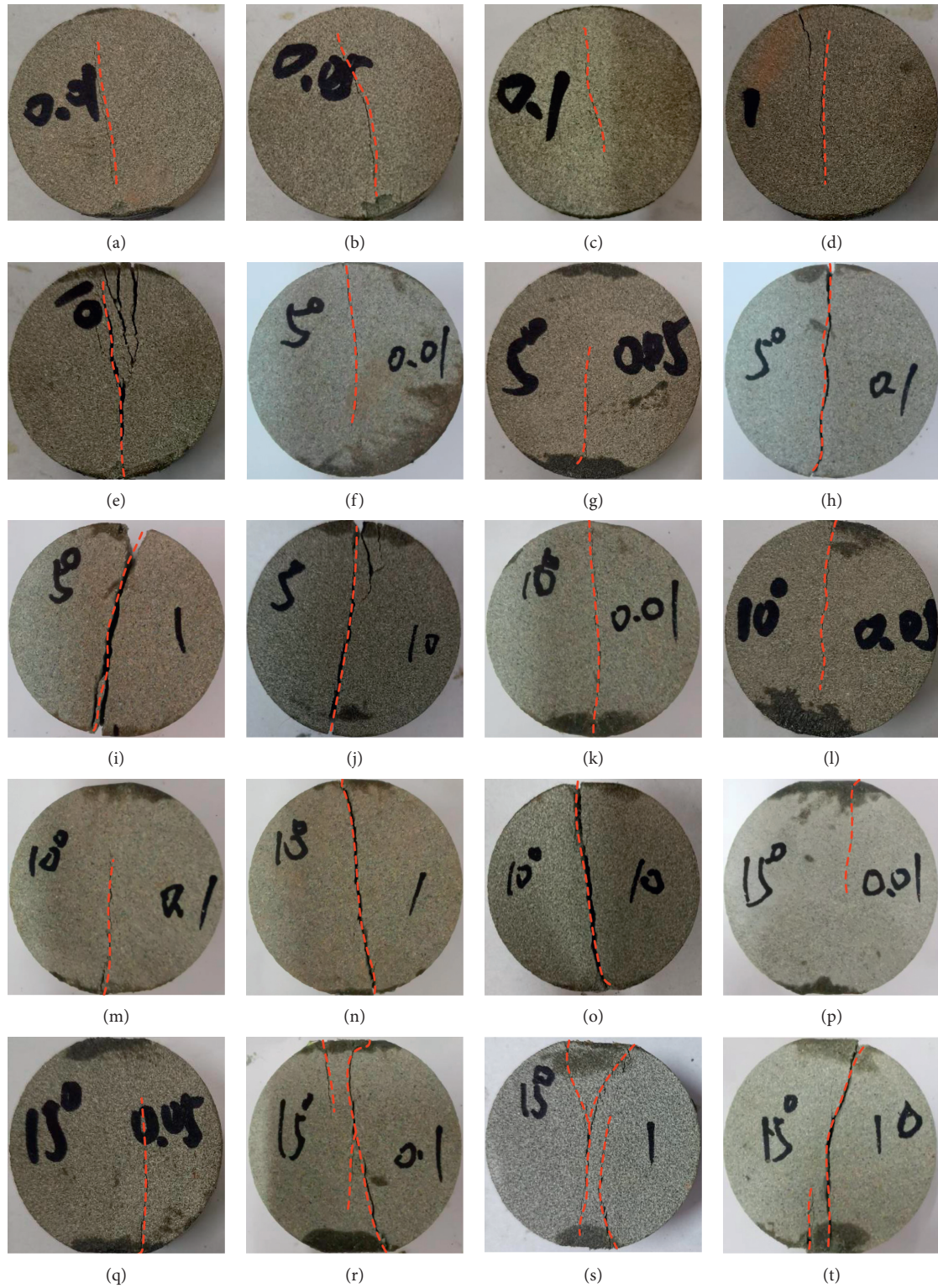
FIGURE 4: Typical failures after indirect tests: (a–e) rock failures at the loading rates of 0.01, 0.05, 0.1, 1, and 10 mm/min, respectively, for the BT tests; (f–j), (k–o), and (p–t) FBT tests with the loading angles of 5°, 10°, and 15°, respectively.
