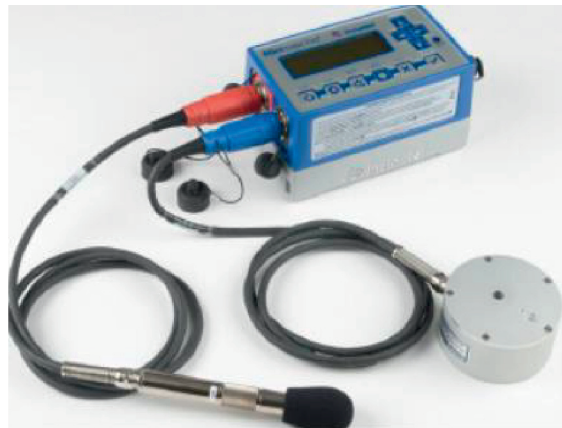
FIGURE 3: Vibration and overvoltage monitor MinimatePro4TM.
