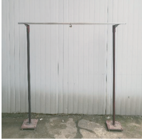
FIGURE 1: Drop hammer lifting device.
