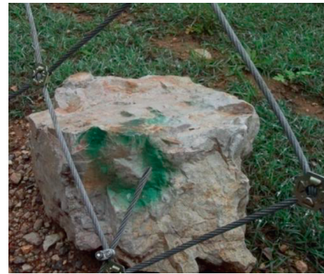
FIGURE 12: Rockfall formed by blasting flyrock.
