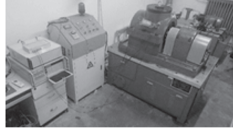
FIGURE 1: Bearing fatigue life test bench.
