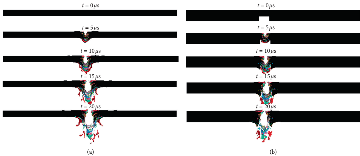
FIGURE 6: Cutting process of the laminate (a) without and (b) with weakening groove.
