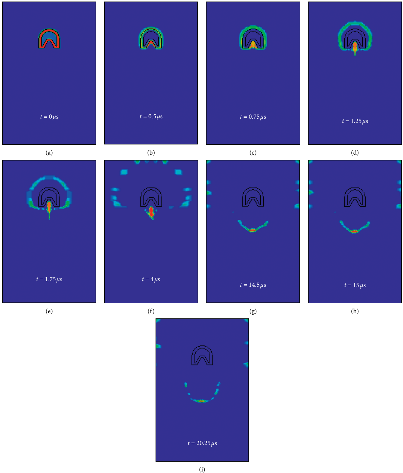
FIGURE 5: Change of shaped charge jet morphology.
