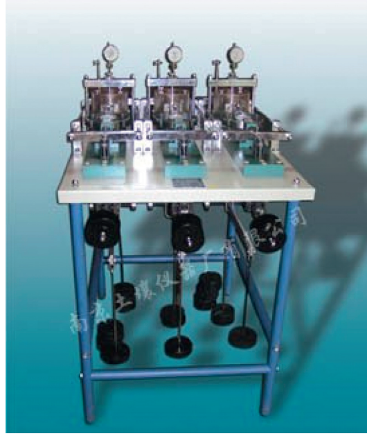
FIGURE 3: The ZLB-1 creep shear apparatus.
