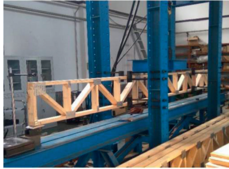
FIGURE 9: Single wood truss in the three-point loading test.
