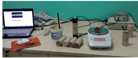
FIGURE 2: Weighing and acoustic testing of rock samples.
