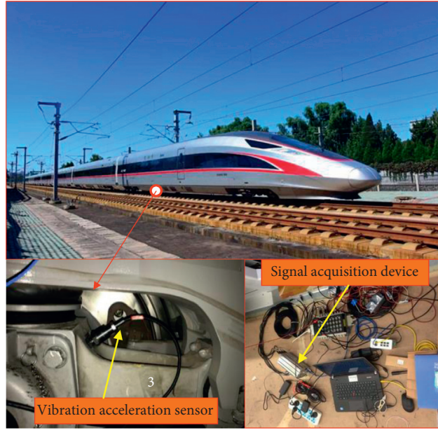
FIGURE 3: Installation of acceleration sensor at the test site.
