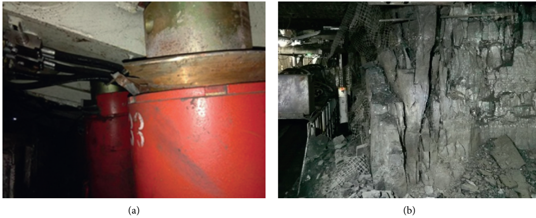
FIGURE 1: Dynamic load hazards in open face area: (a) shield collapse from roof fall; (b) face failure from excessive roof-to-floor closure.
