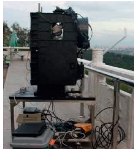
FIGURE 2: Large-load motor turntable.
