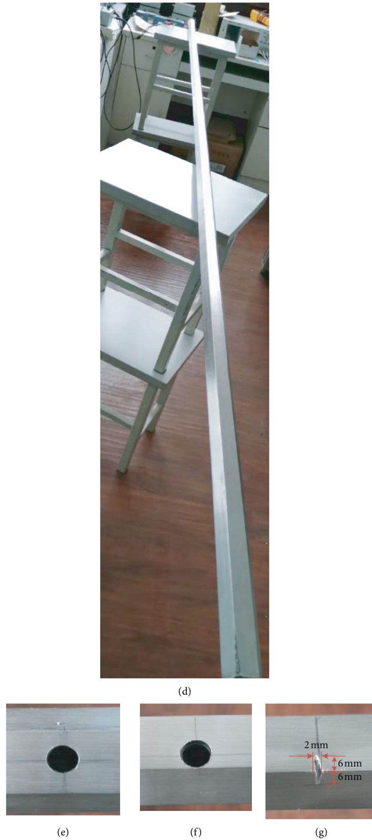
FIGURE 16: Experimental setups: (a) experimental platform; (b) the configuration of a ring of PZTs with the size of 25\text{ mm} \times 5\text{ mm} \times 0.5\text{ mm} ; (c) a ring of PZTs with the size of 30\text{ mm} \times 5\text{ mm} \times 0.5\text{ mm} ; (d) experimental specimen of hexagonal pipes; (e) circular hole damage located in the center of a surface plane; (f) circular hole damage near the edge of a surface plane; and (g) slot damage located at the edge with its dimensions.
