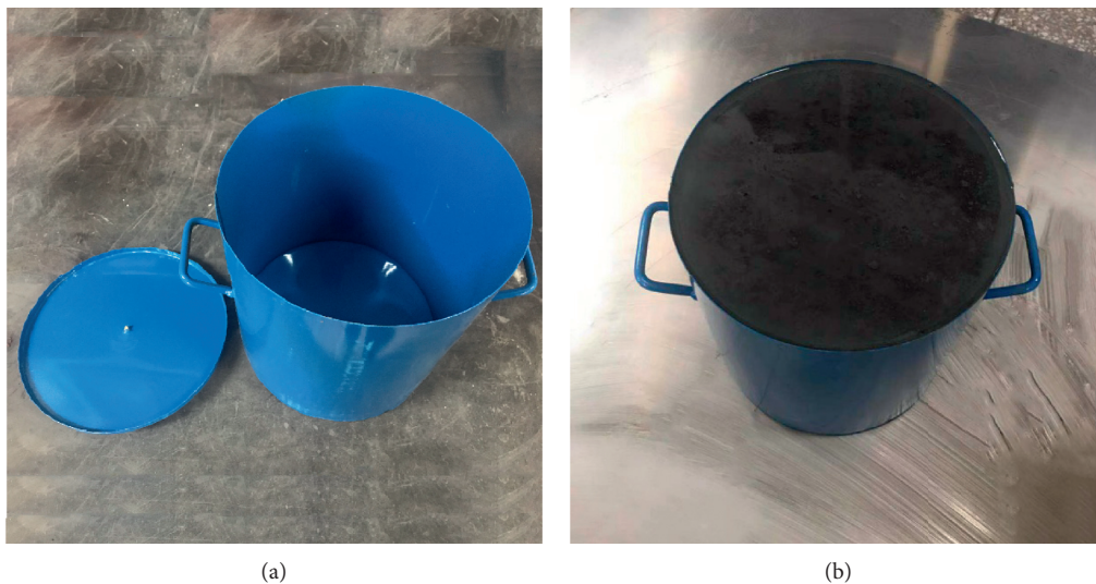
FIGURE 4: Graph of bleeding rate test. (a) Measuring device. (b) Bleeding rate measurement.
