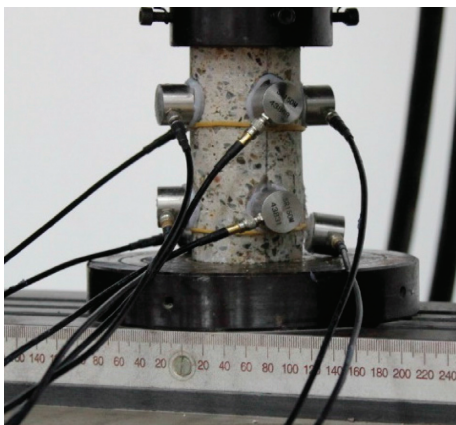
FIGURE 2: Loading device and arrangement of AE sensors.
