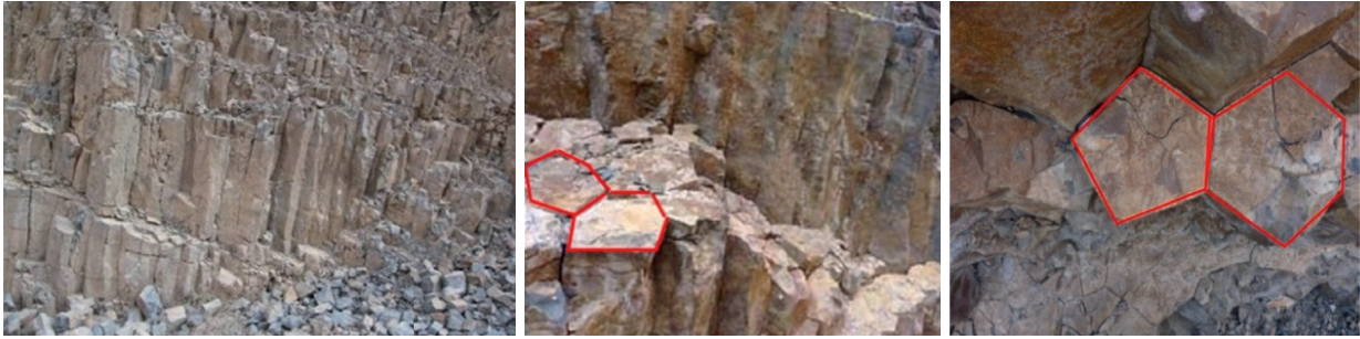
FIGURE 1: Columnar jointed rock mass in the dam site area of the Baihetan hydropower station.
