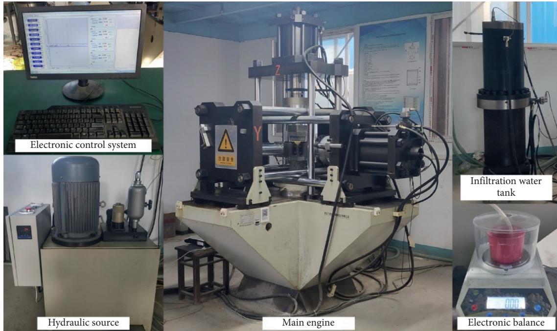
FIGURE 4: The true triaxial test system for determining the rock fracture seepage.
