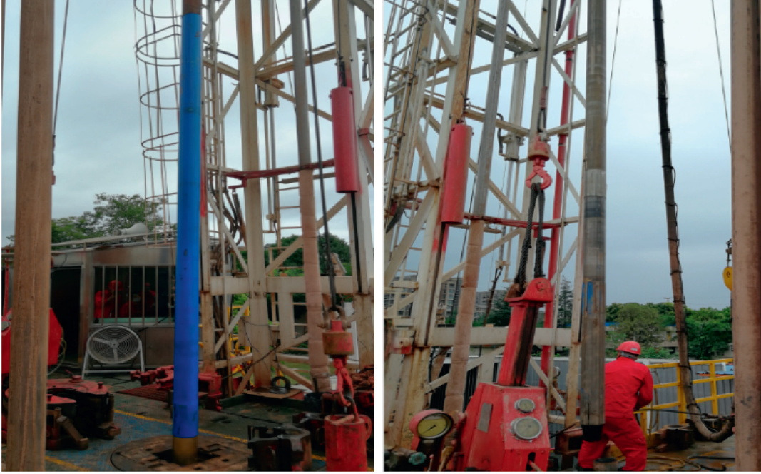
FIGURE 4: Tool tripping in and tripping out.
