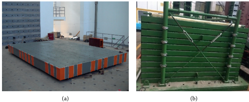
FIGURE 3: Shaking table and layered shear deformation model container. (a) Specimen-mounting table (4 × 6 m). (b) Model container (2 (length) × 2 (width) × 1.3 (height) m × 0.1 (wall thickness)).
