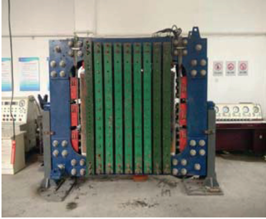
FIGURE 1: Multifunctional testing machine for rock and soil.
