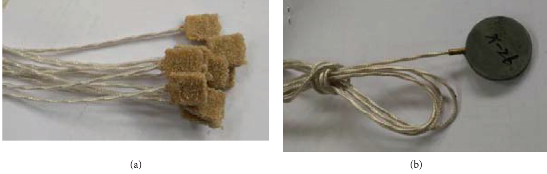
FIGURE 5: Stress and strain sensors in the model test samples. (a) Strain sensors. (b) A PVDF stress sensor.
