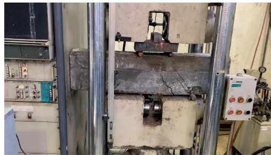
FIGURE 10: Cracks created in a specimen of the concrete beam reinforced with the carbon-basalt hybrid bar.
