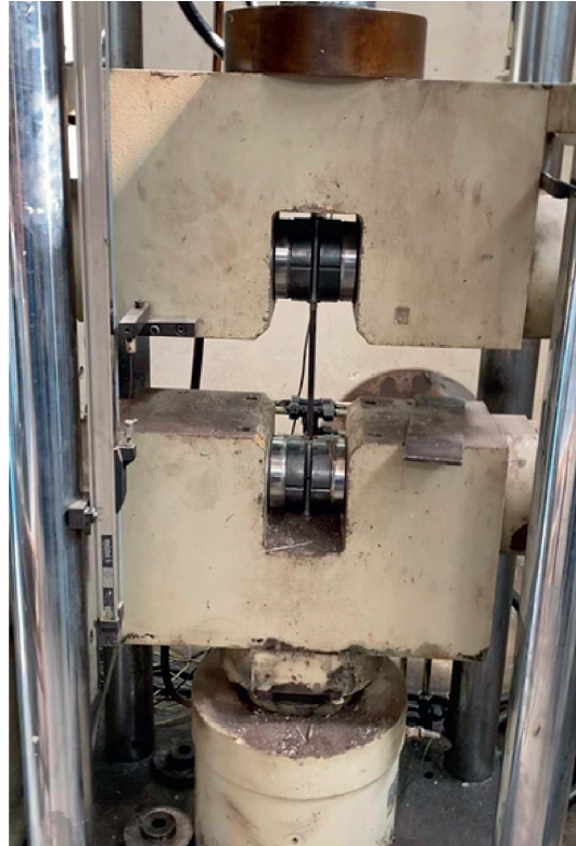
FIGURE 3: Tensile test of hybrid composite bars.
