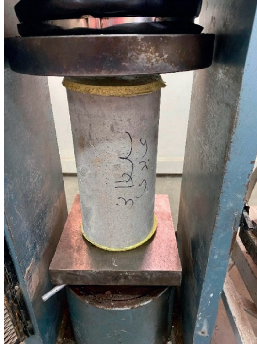
FIGURE 5: Measuring compressive strength of concrete using standard cylinders.
