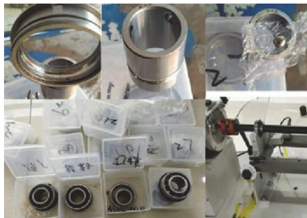
FIGURE 6: SER205 fault bearings.
