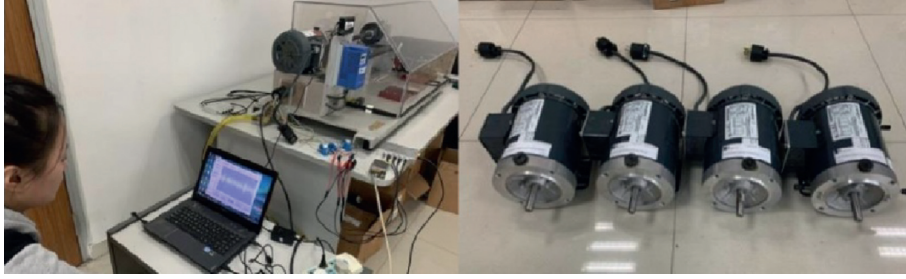
FIGURE 7: Motor fault data collection and fault motors.
