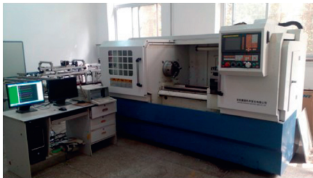
FIGURE 2: The physical diagram of the multi-information data acquisition system of tool wear condition of CNC lathe.
