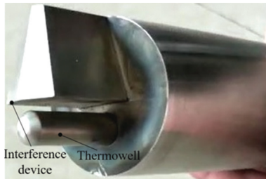
FIGURE 27: Thermowell with interference device.
